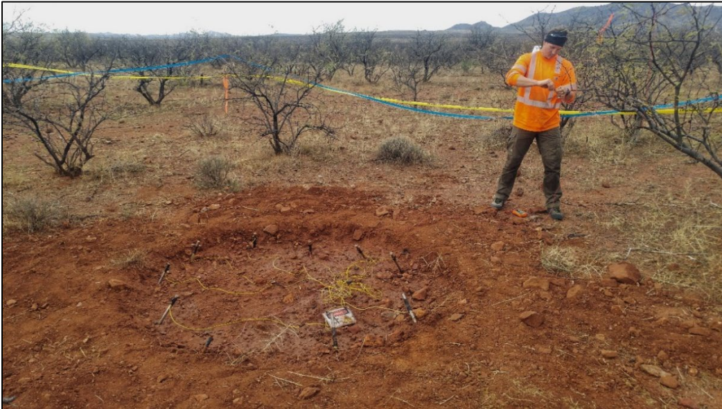
Figure 4. Example of a temporary current injection point showing a small diameter hole with several steel rods wired together in a saltwater solution. The entire site is reclaimed after about 20-30 minutes of transmit time.
