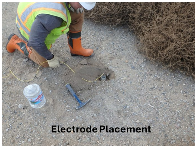
Figure 6: Installation of components of a Mageto Telluric geophysical survey.
