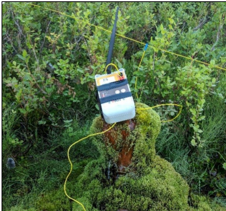
Figure 2. Receiver node measures small voltages with no associated electrical risk.
