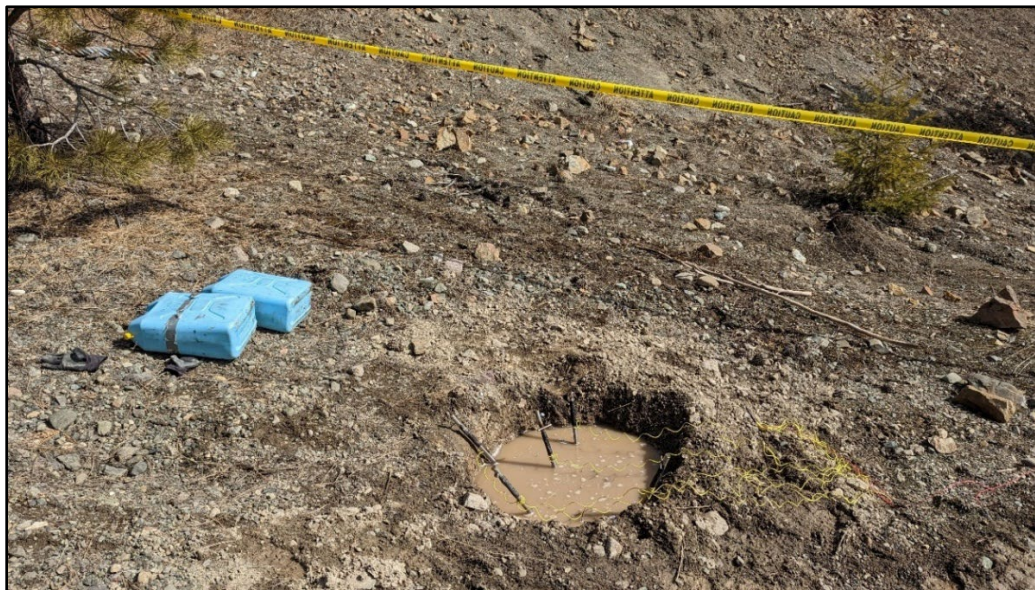
Figure 4. Example of a temporary current injection point showing a small diameter hole with several steel rods wired together in a saltwater solution. The entire site is reclaimed after about 20-30 minutes of transmit time.
