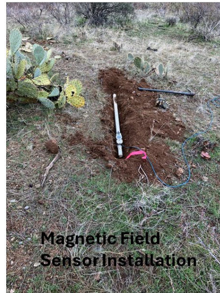
Figure 6: Installation of components of a Mageto Telluric geophysical survey.
